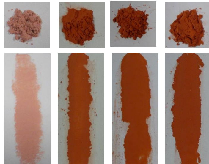
TiO 2 + untreated red iron oxide MAKIBEADS 2 + ASL- red iron oxide MAKIBEADS 2 + OTS-red iron oxide MAKIBEADS 2 + MST-red iron oxide
